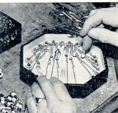
Assembling the action. In an instrument of this size— a 40 key "Anglo" model—there are over 400 parts in the action alone.
